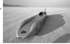
computational fluid dynamics, which has enabled the car to obtain a very low coefficient of drag of only 0.174 and a CdA value of only 0.153 m<sup>2</sup>. Some JCB!
