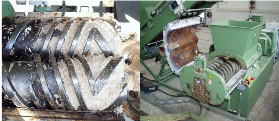
Figure 1: Open twin-screw extruder with material inside (left), whole extruder opened (right) at ATB
