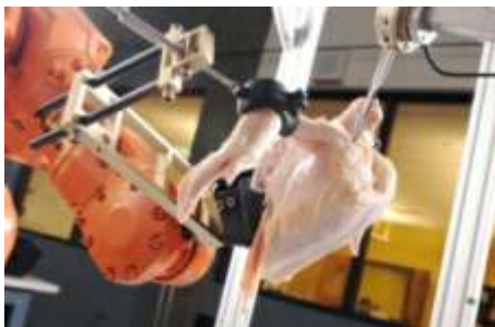
A robotic system used in the Intelligent Cutting and Deboning project prepares to slice through the shoulder joint of a chicken. (GT Photo: Gary Meek)
