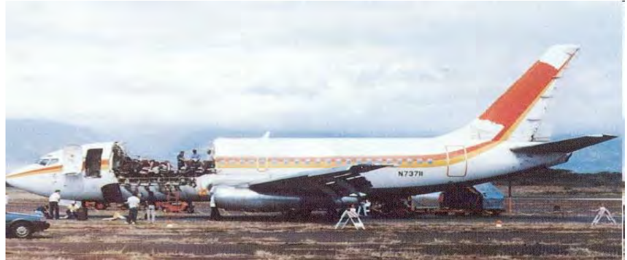
Hawaii 1988, lap joint failure
